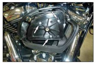
3. Loosen the three air filter retaining bolts as shown.
