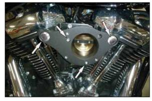
9. Using the two provided crankcase breather bolts; install the back plate onto the vehicle. Do not tighten bolts at this time. Make sure O rings do not fall out during this operation. Install the two allen bolts and tighten all bolts at this time. **NOTE: Apply one drop of the provided thread locker onto the bolts.**
