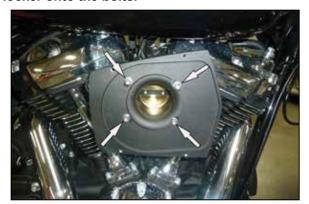
10. Install the air scoop base gasket and base plate with the provided hardware. Slightly tighten at this time. Using the air filter cover clock the filter base in position then finish tightening filter base plate. **NOTE: Apply one drop of the provided thread locker onto the studs.**
