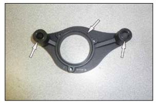
7. Install three of the O rings provided onto the back side of the  $K\&N^{\otimes}$  back plate as shown.
