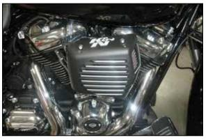
11. Install the K&N $^{\ensuremath{\mathbb{R}}}$  air filter and filter cover with provided bolts.
