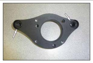
8. Install the remaining two o rings onto the front of the back plate as shown.
